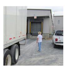
should assess overhead clearance (overhangs, drain pipes, power lines, etc.) as well as the width of the area to be backed into. If conditions change while backing, the driver should get out and look again. GOAL—it only takes a few minutes!
