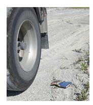
Drivers can create their own landmark by placing a glove on the ground at the first point they want to back to.
