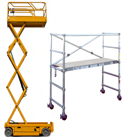
Scissor lift (left) and mobile scaffold.
