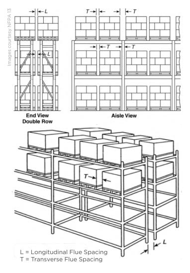
There are two types of flue spaces - transverse and longitudinal.
