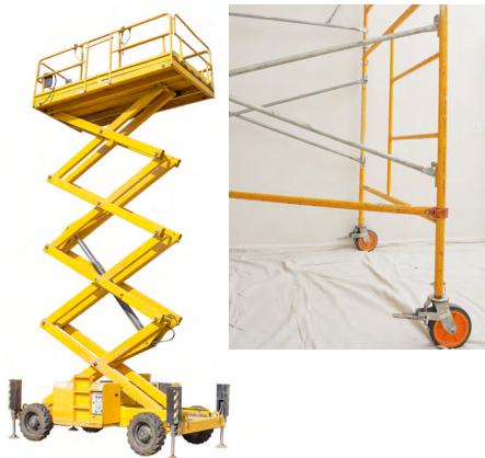
Scissor lift (left) and mobile scaffold.
