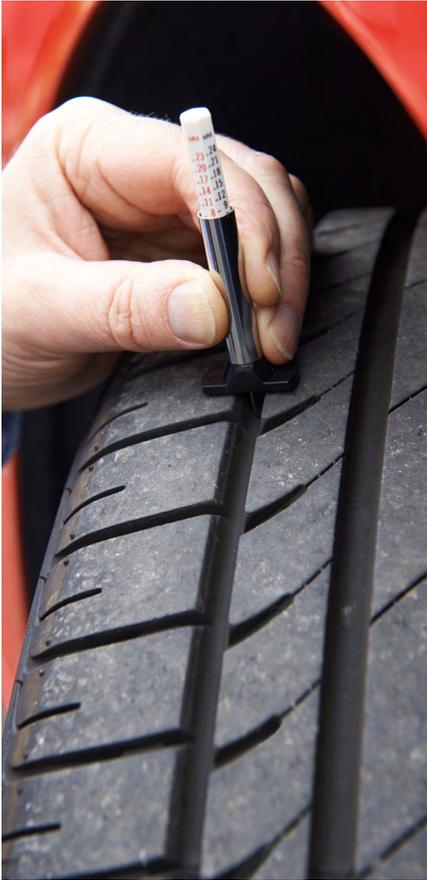
Tire inspection and proper inflation are critical in preventing rollovers. NHTSA found 15-passenger van tires to be mis-inflated by 25% or more in 74% of cases.<sup>2</sup>
