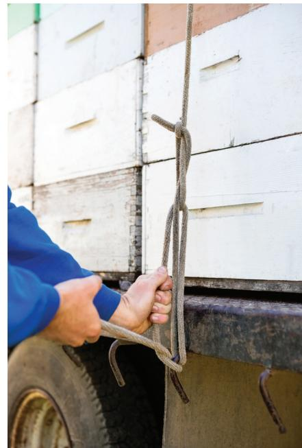
On flatbed trucks or trailers, there should be at least one tie-down for each 10 feet of cargo.
