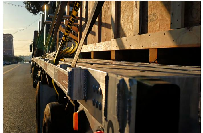
**Indirect cargo securement** is a tie-down that goes from an anchor point on the vehicle, through, over, or around the article of cargo, and then attaches to another anchor point on the other side of the vehicle. Indirect tie-downs create a downward force that increases friction between the cargo and the deck of the trailer.
