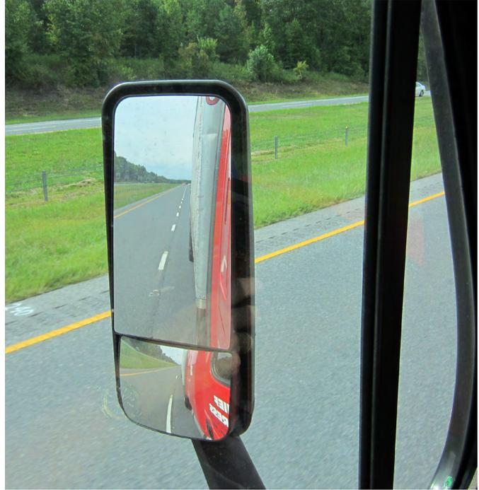
Ensure mirrors are adjusted to minimize blind spots.
