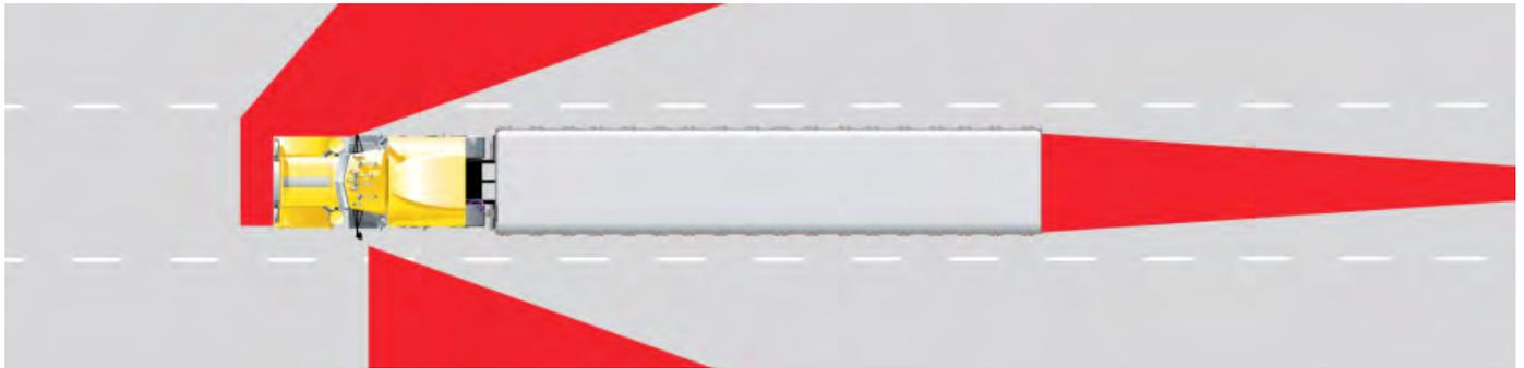
Truck blind spots (red) vary depending on the design of the truck and mirrors. Drivers need to ensure other vehicles are not in these blind spots before changing lanes.
