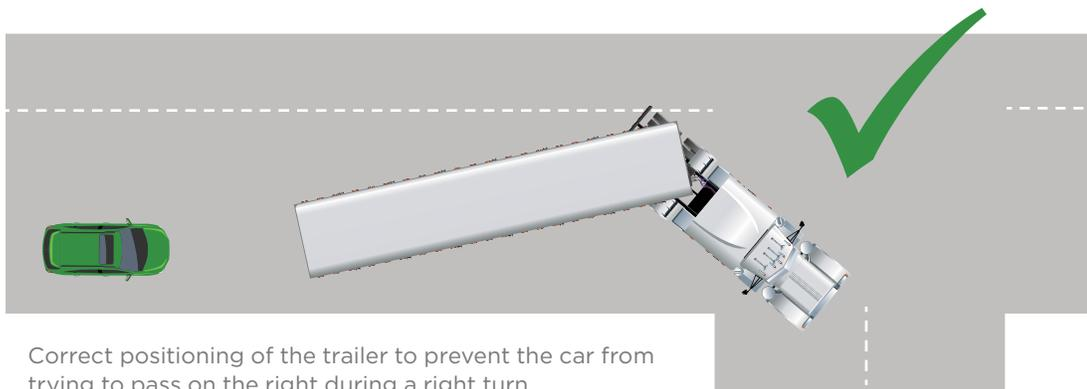
Correct positioning of the trailer to prevent the car from trying to pass on the right during a right turn.
