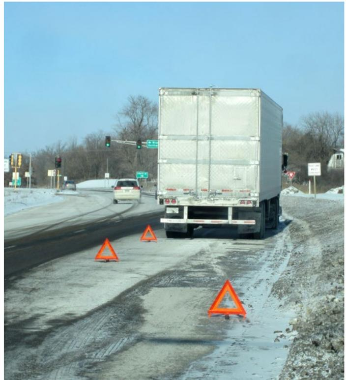
**The driver in the photo did not set out their triangles correctly. Refer to the diagrams below for proper placement.**
